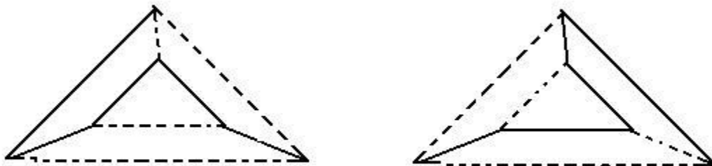
These two spanning trees of the right triangular prism define the same unfolding
